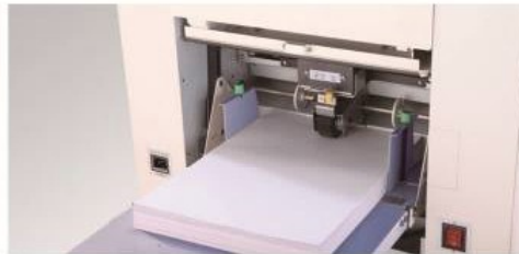
Innovative design of paper feeding by double rollers which is much more stable. Simultaneously feed paper to guarantee one page input only once.
